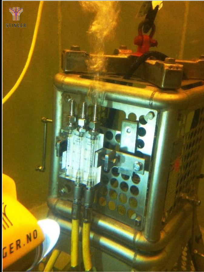
Seabed Gas leakage simulator
